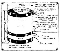
fig. 5. A real shortwave receiver for pennies that actually works. Thousands of would-be hams built this simple set from the pages of "Short Wave Craft" during the "thirties" and were thrilled with world-wide reception.
